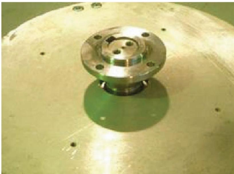
RETIRADAS LAS PLACAS ANTICAÍDA DESMONTAR EL BUJE DEL EJE
